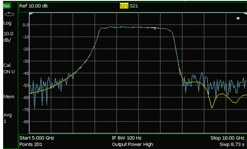
Figure 6. Measurement comparison of a 13-GHz band pass filter response using the High Output Power setting (yellow) and the Low Output Power setting (blue) on FieldFox
